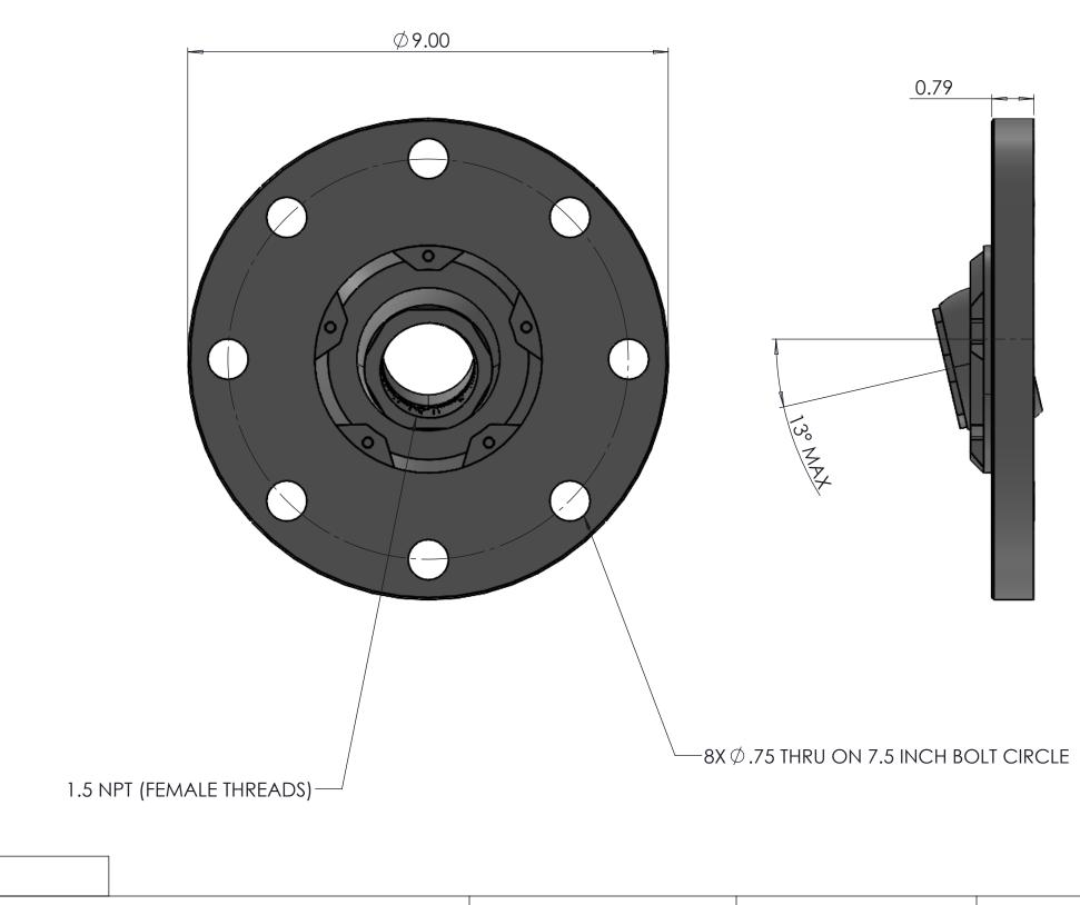
TITLE: SWIVEL MT 9IN DIA. FLANGE WITH 1.5 NPT BALL MODEL NO.: SWVL-15 P/N: SWVL-15,9AXX DWG NO.: 418-0300 MATERIAL: GF POLYPROPYLENE
