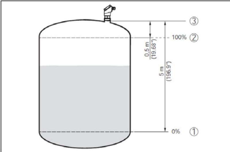
Fig. 16: Parameter example, Min./max. adjustment
