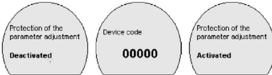
With activated protection of the parameter adjustment, the individual menu items can be selected and displayed, however the parameters can no longer be modified.
