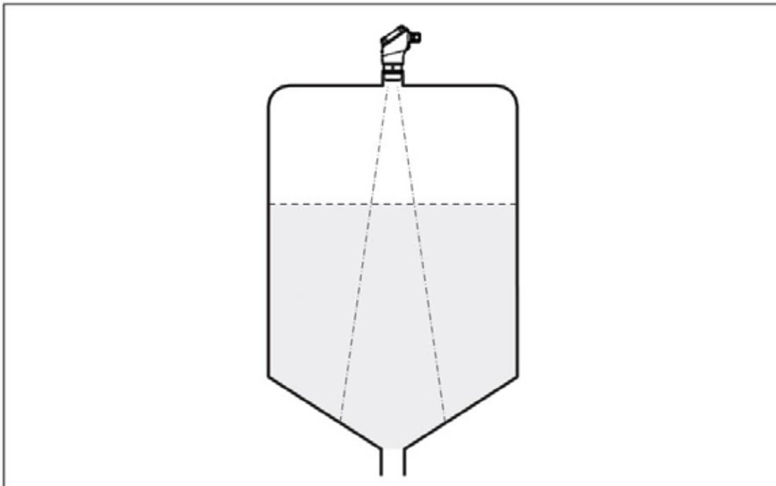
*Fig. 7: Mounting the radar sensor with conical bottom*
