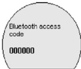
For instruments without Bluetooth function, this menu item displays *“Instrument without Bluetooth”*.
