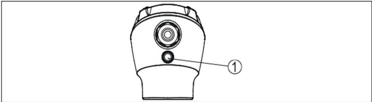
*Fig. 4: Polarization Position*
