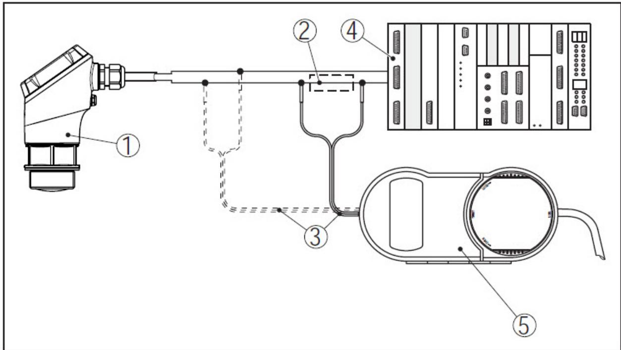
Fig. 3: Connecting the PC to the signal cable
