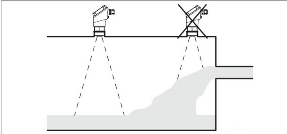
*Fig. 8: Mounting the radar sensor away from the fill stream.*
