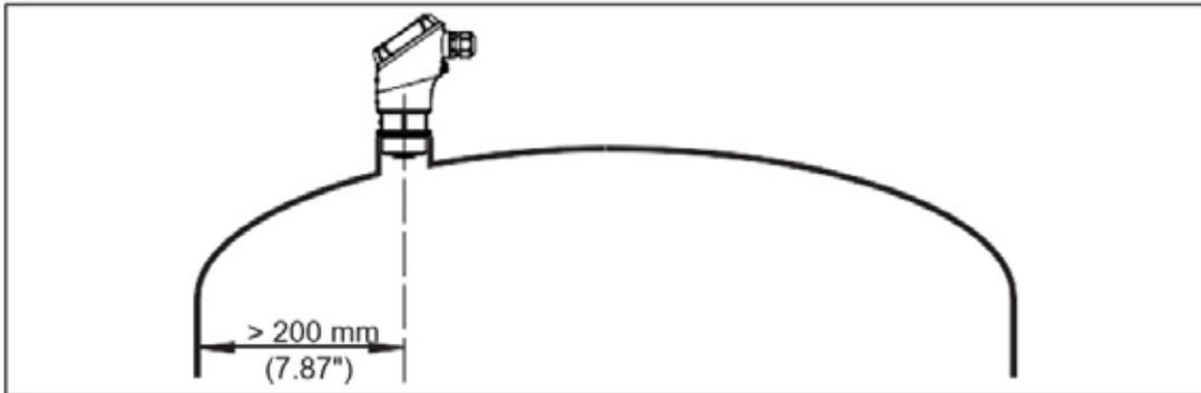
*Fig. 6: Mounting the radar sensor on round vessel tops*
