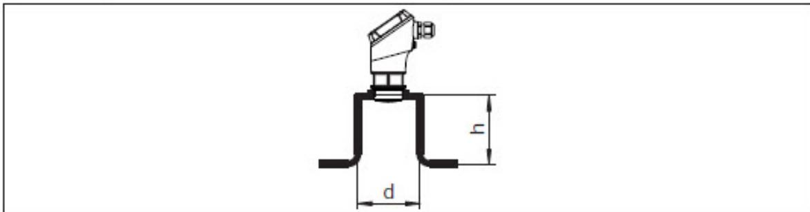
*Fig. 10: Mounting the radar sensor with stand pipes*
